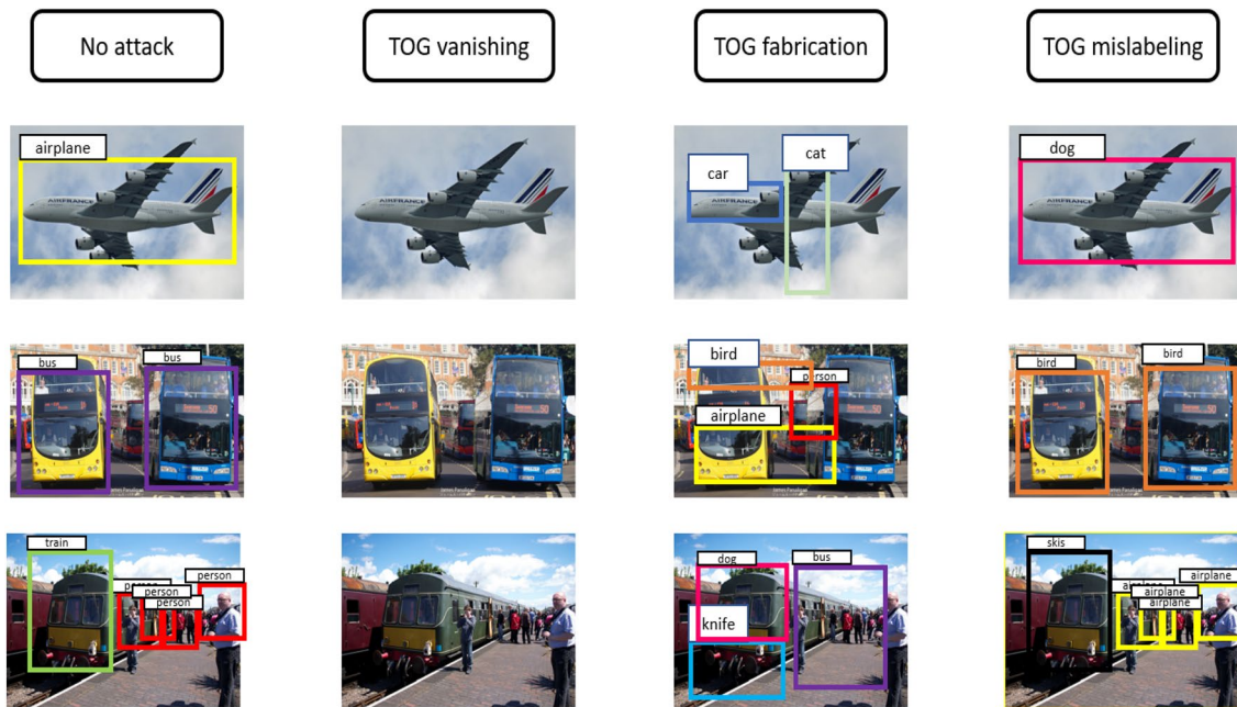
Fig. 6 The effects of targeted attacks on the recognition performance of the object detector
