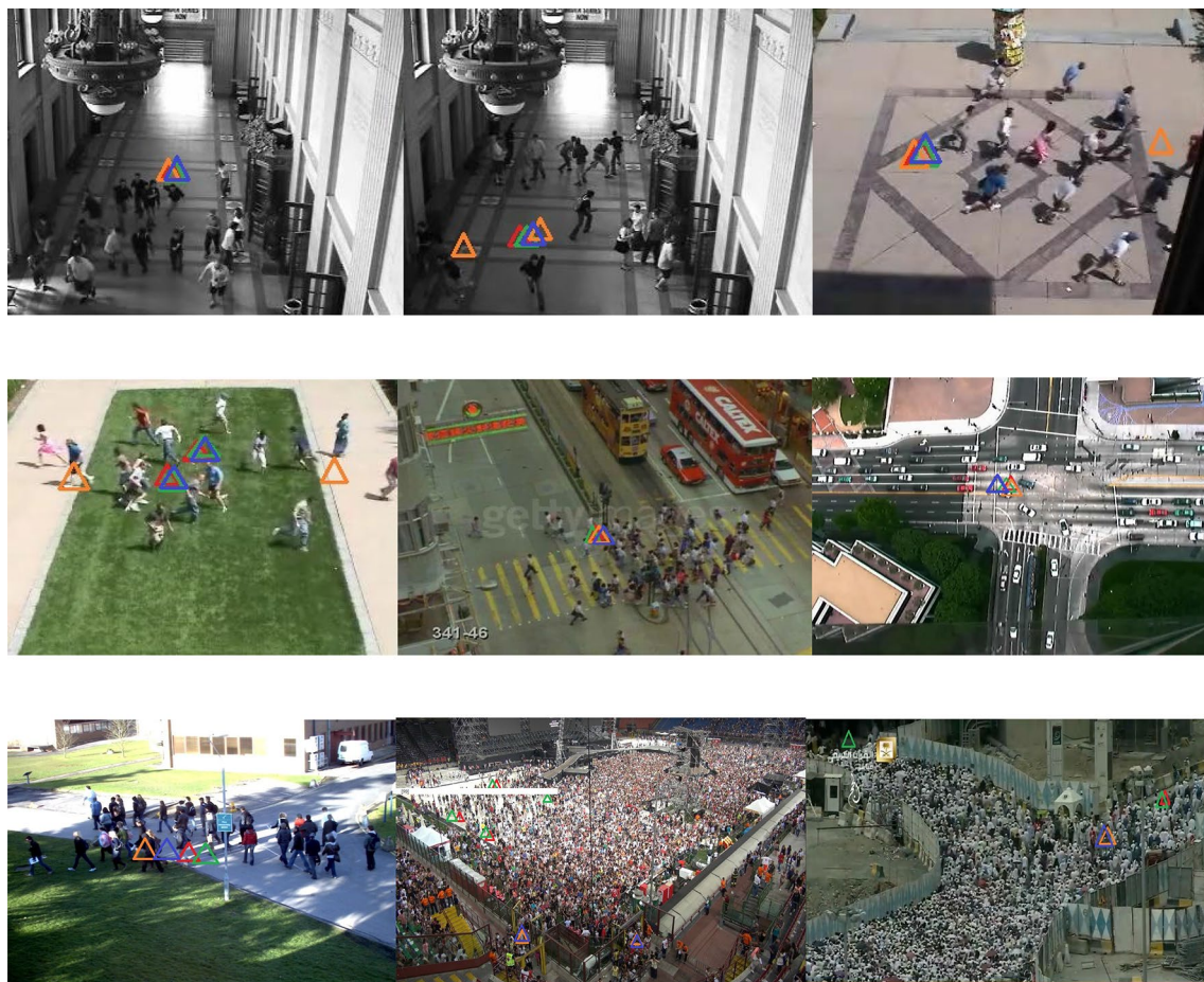
Fig. 27 Divergence localization comparison with state-of-the-art methods. Legends: red triangle [7], green triangle [8], orange triangle our method, blue triangle ground truth. The top two rows show divergence localization at low-density scenes. False divergent center
