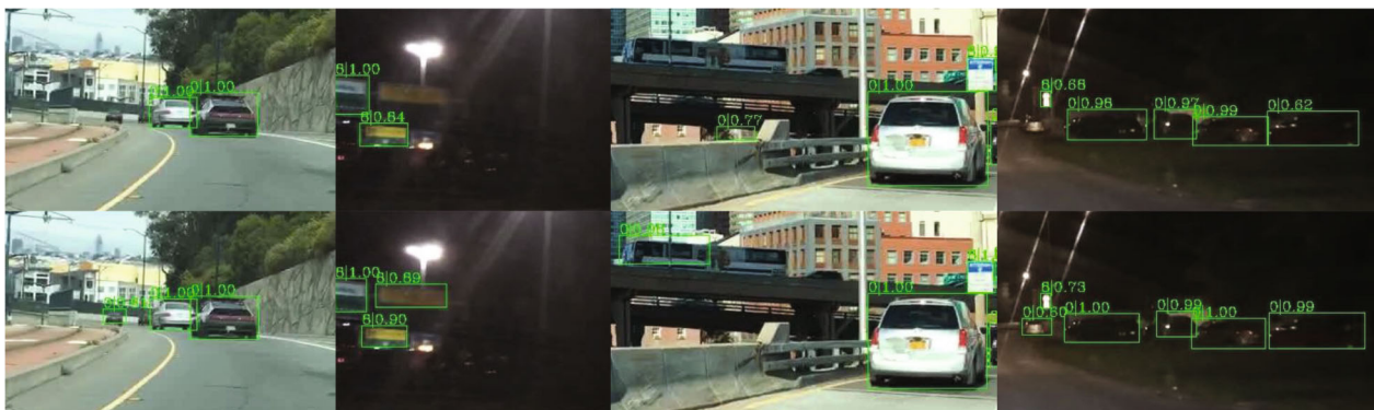
Fig. 8 Detection results of the baseline and proposed algorithms on the BDD validation set. The first row shows the detection results of RetinaNet, whereas the second row shows the results of RetinaNet+CDFL
