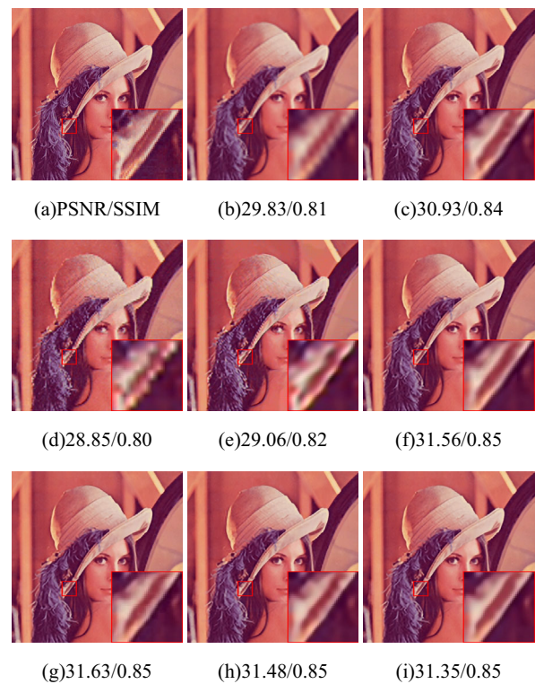
Fig. 11 Super-resolution comparison on lena image ( \times 4 ): a original, b bicubic, c NLFIBP, d RFI, e LPRGSS, f MMPM, g FSRCNN, h DLD, i proposed
