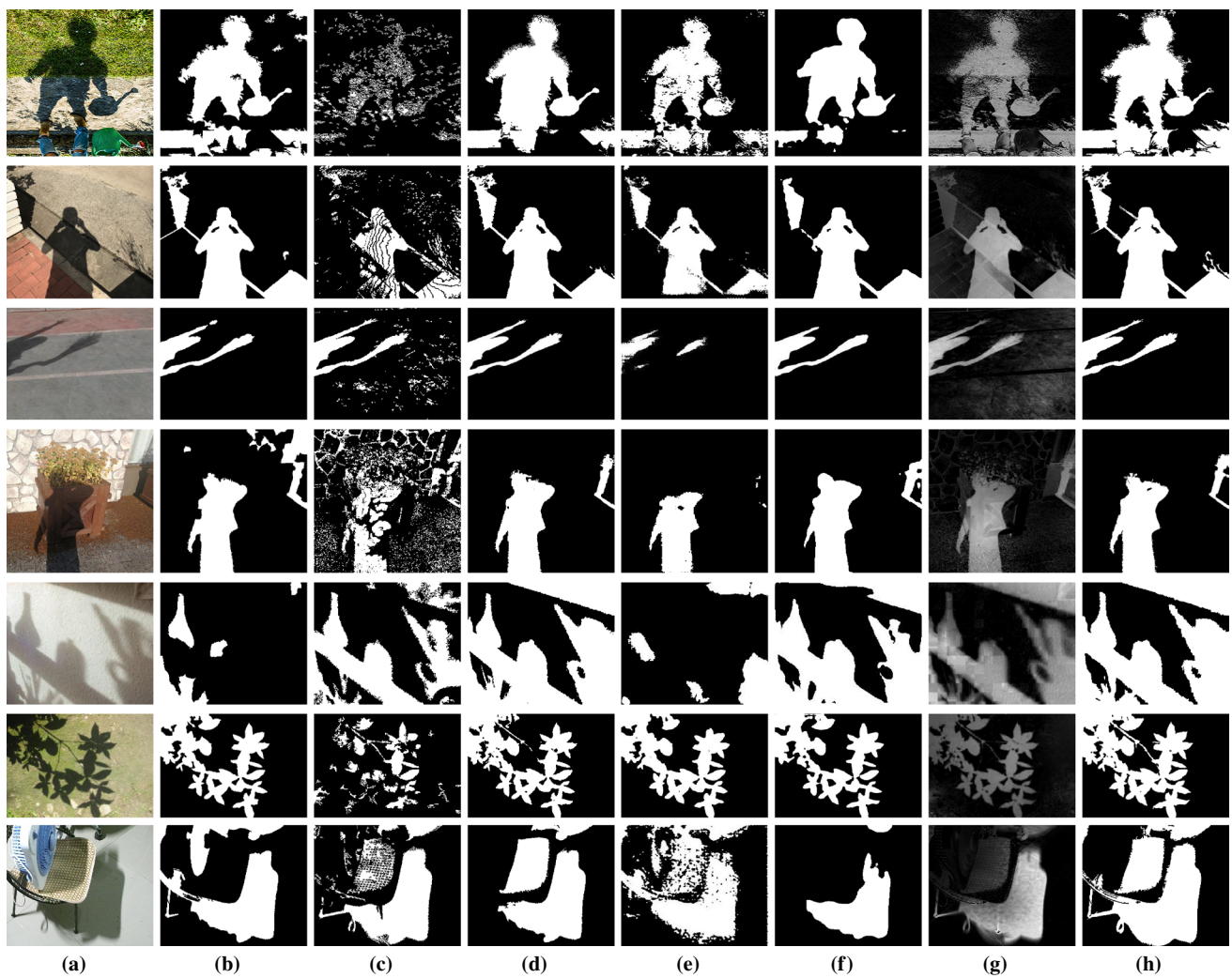
Fig. 8 Visual comparison on shadow detection results. From left to right are a input images, b results of Guo [15], c results of Xiao [42], d results of Zhang [48] incorporating user interactivity, e results of Wang [37], f results of DSC [17], g our refined shadow confidence maps and h the binary results based on g
