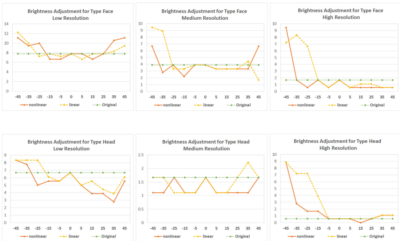
Fig. 8 Brightness adjustment. The x-axis and y-axis show the adjusting amount of \beta (%) and HTER error (%), respectively
