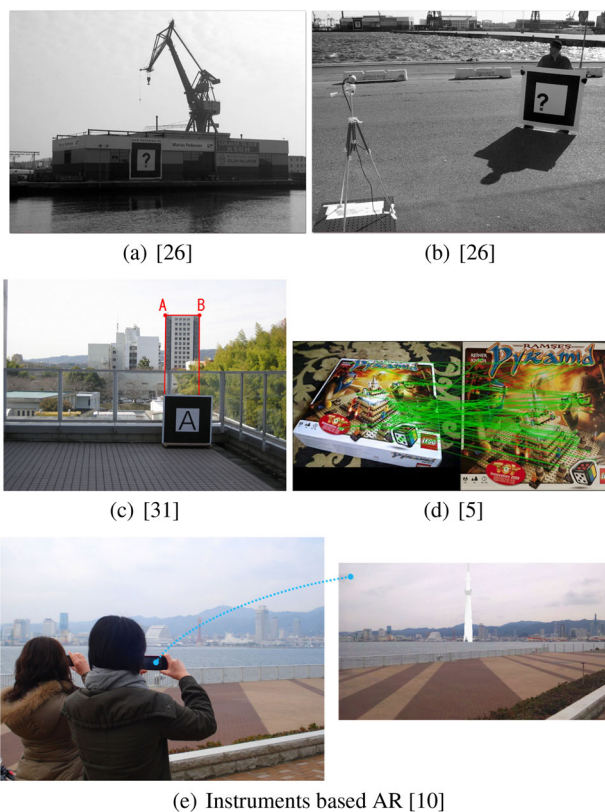
Fig. 1 Different AR approaches. a, b and c Artificial marker-based AR; d Natural markers AR-based; e sensor-based AR
