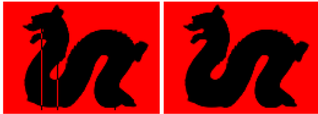
Fig. 5 Slice from the distance field of the dragon model. Using only one direction (left) may lead to wrong inside–outside classifications due to imperfect models or edge cases in the intersection routines. Using six rays can fix these small errors (right)
