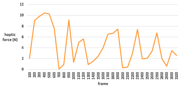
Fig. 16 Haptic force measured when the hook contacts the fat tissue during electrocautery simulation
