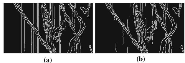
Fig. 6 Preprocessing step for the abnormal event detection problem. From the visual rhythm, edges are found by Canny detector (a) to represent directional information of the trajectory; but the background produces a noisy pattern as vertical lines that is removed by using opening morphology (b) with a vertical line as the structuring element
