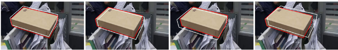
Fig. 10 The influence of different initial camera pose for the Simple Box model, where the white lines denote the initial camera poses, and the red lines denote the tracking results
