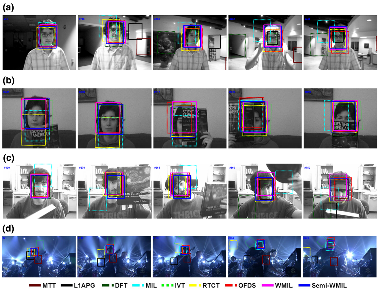
Fig. 8 Screenshots of some sampled tracking results for tested sequences: DavidIndoorOld , Occlusion1 , Occlusion2 and Shaking (from top to bottom). Figure best viewed in color and line style. a DavidIndoorOld , b Occlusion1 , c Occlusion2 , d Shaking
