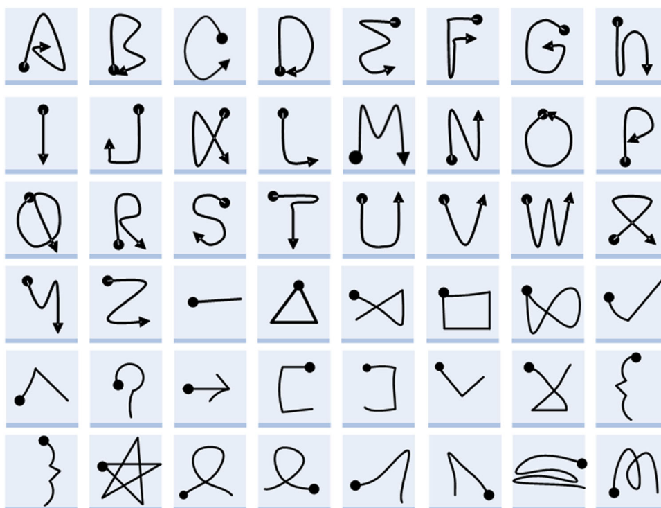
Fig. 7 Gesture vocabulary. The beginning of a gesture is indicated by a solid dot
