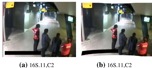
Fig. 8 a Presence of the barrel distortion in C2 is more clearly visible towards the left edge of the frame where the vertical structure appears to be bent outwards and b distortion-corrected frame
