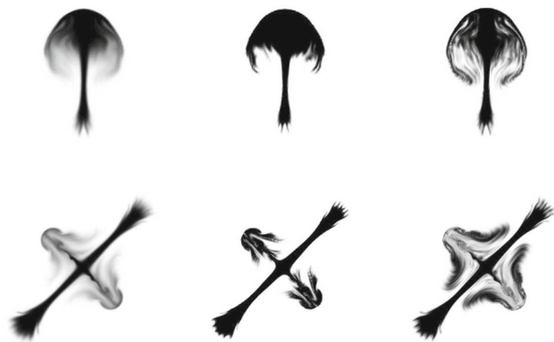
Fig. 6 Smoke simulation with fire simulation using DBCM method. Fuel and temperature field were used to simulate the fire. DBCM advected the density, fuel and temperature field simultaneously with the same mapping function and captured rich details of the distribution of these physical variables (visualized as smoke and fire). N_c was set to 256 for \chi and N_f was set to 256 for \chi^R for DBCM method
