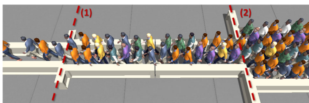
Fig. 6 Two bottlenecks scenario. We simulate and compare crowd behavior at two narrow bottlenecks, which are marked with red dotted lines . Bottleneck (1) is barely wide enough for one person to pass through; bottleneck (2) is about twice that width and allows two agents to pass through it at a time. The result from collision-avoidance-only simulation results in an arch-shaped arrangement of agents in the crowd (highlighted with a yellow circle ), which causes congestion at the bottleneck. Our method breaks the congestion by allowing the agents to push one other in congested conditions
