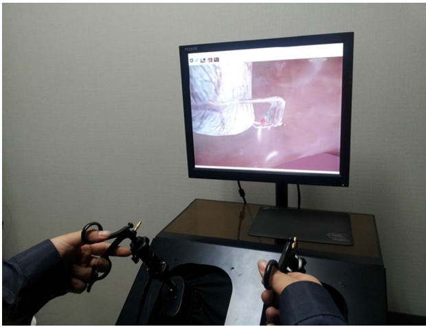
Fig. 7 Integrated laparoscopic surgical training simulation system. (NT Research Co.) [33]
