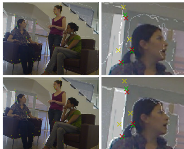
Fig. 2 Camera calibration: The perspective projection parameters are obtained by minimizing the distance between RGB points and the perspective transformation T_\theta of the projected depth points. In the figure, the depth gradients image is superimposed on the color image before (top) and after (bottom) registration. The yellow marked points ( q_i ) are matched to the green ( p_i ) by the user. After registration procedure the new position of the yellow points is marked in red
