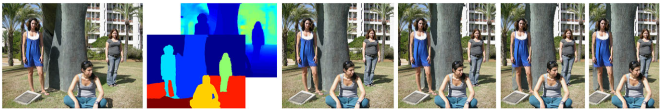
Fig. 1 Segmentation and retargeting using depth: (from left to right) color image, depth image and our automatic segmentation using color and depth overlaid, color image retargeted by 20%, 30%, 40%, and 50%
