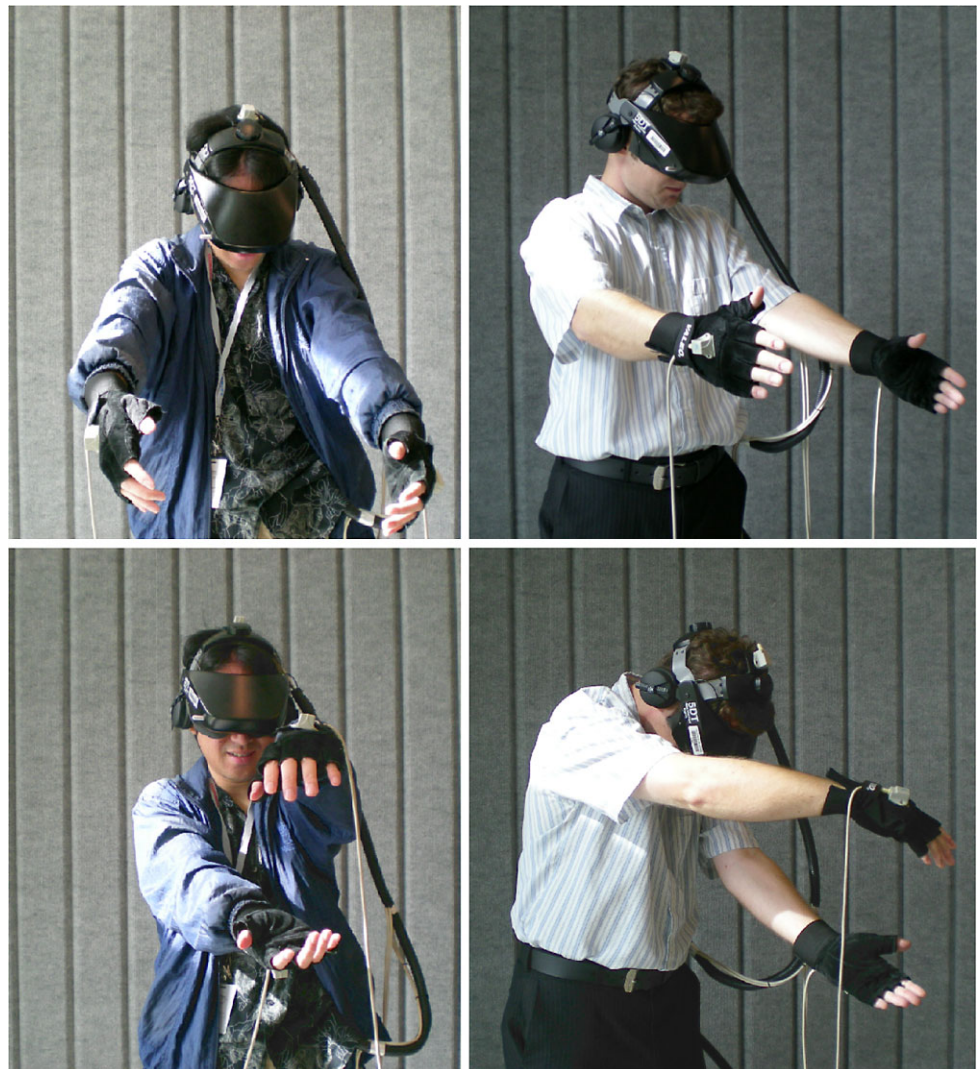
Fig. 1 VR users demonstrate areas of hand visibility for a 40° HMD: horizontal ( top ) and vertical ( bottom ). Both hands and head are tracked in 6 degrees-of-freedom. In order to see their hands, users sometimes have to assume very uncomfortable poses ( bottom right )
