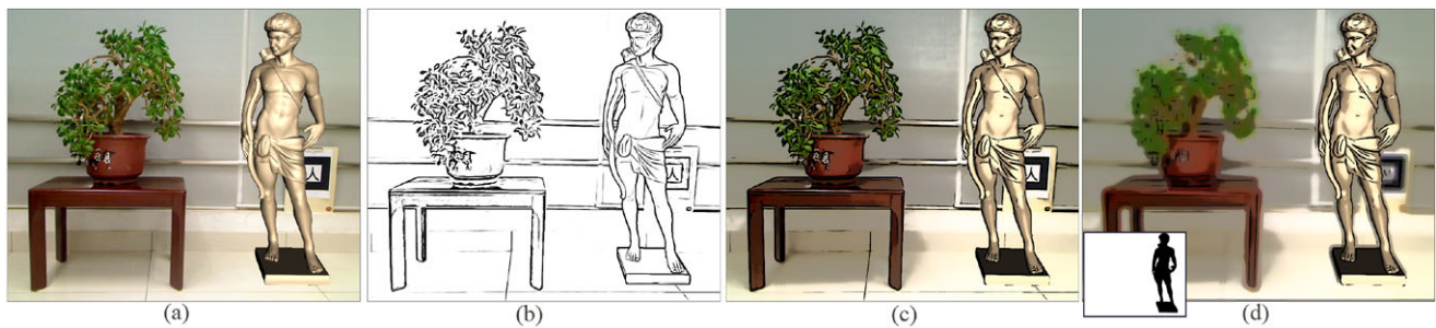
Fig. 1 Stylization for augmented reality: (a) is a conventional AR frame containing a virtual model of sculpture, in which there exist the apparent distinctions between real and virtual contents; (b) is the effect
