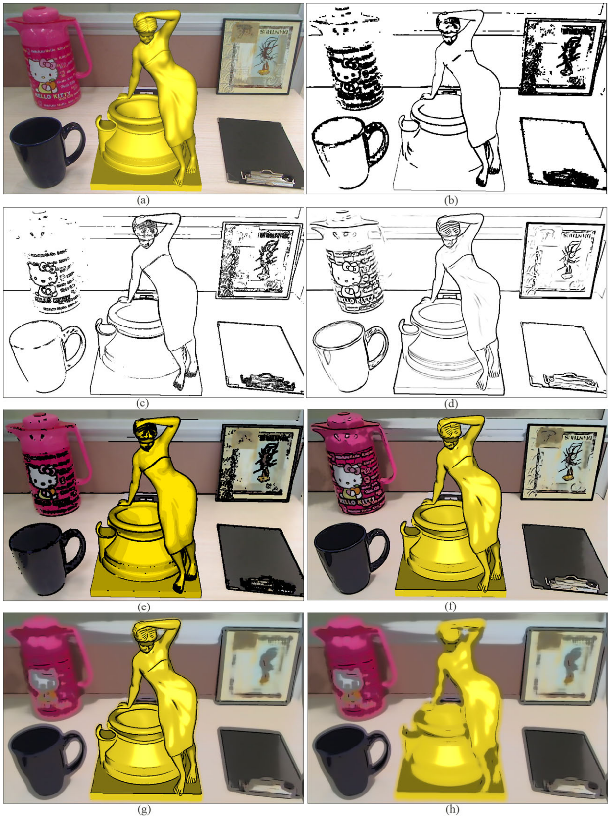
Fig. 7 Comparison with other stylized AR techniques. (a) Conventional AR scene, in which the statue of a woman is virtual. (b) “Sketch-like” stylization by [10]. (c) Edge detection by [4]. (d) Line drawing
