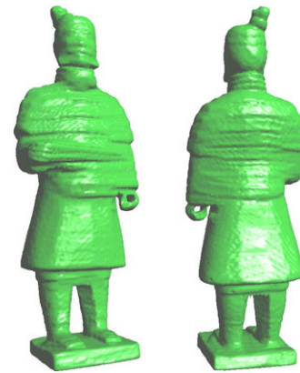
Fig. 5 Two views of the visual hull mesh of the Soldier object extracted from 8-level octree structure
