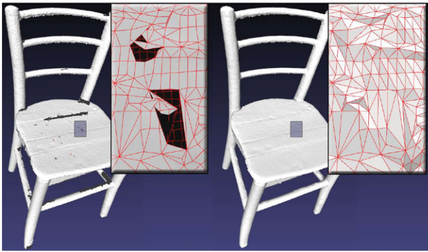
Fig. 1 The raw model of a chair was produced by merging a set of views acquired through laser scanning ( left ). The same model was processed through the algorithm described in this article to become the watertight surface of a polyhedron ( right ). Raw model courtesy of Aim@Shape
