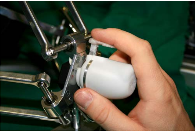
Fig. 7. Prototype of one DoF gripping force master device
