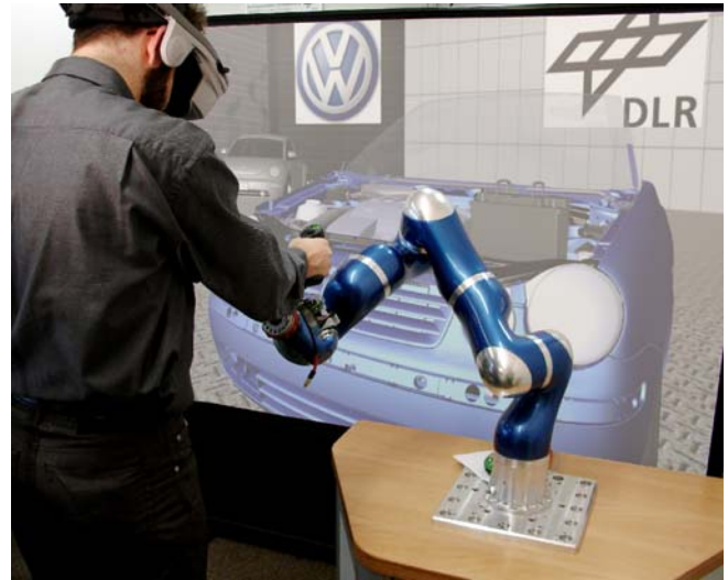
Fig. 6. DLR handcontroller on basis of the DLR LWR3
