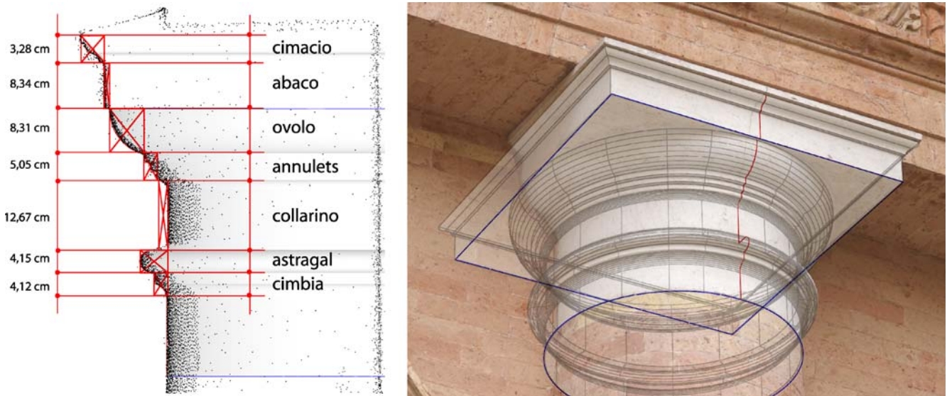
Fig. 19a,b. The primitive instantiated on the point cloud. On the left b , the vertical profile with dimensional information. On the right a , the primitive projected on a photography oriented on the point cloud
