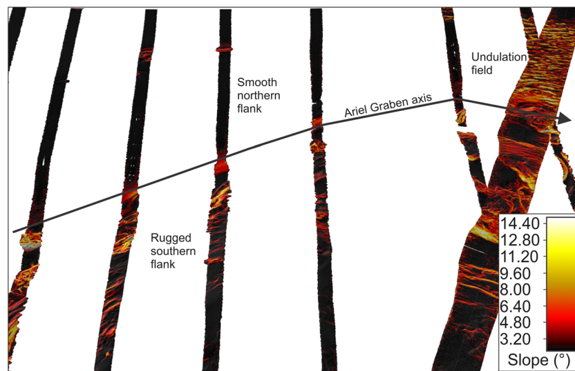
Fig. 7 3D perspective view slope map for the Ariel Graben looking south to north from the Dana plateau across the Ariel Graben. The strips of data reflect the slope of the seafloor as calculated from the bathymetry data from the same area. Note the difference in slope and relief between the northern and southern flanks of the Ariel Graben. The northern flank is
