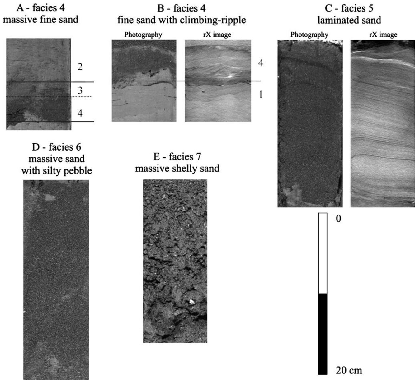
**Fig. 2** Photography and X-ray images of the sand facies identified in the Golo turbidite system. *a* Massive sand or graded sand showing various dynamic structures. *b* Fine sand with climbing ripples. *c* Laminated graded sand. *d* Massive sand. *e* Coarse homogeneous shelly sand
