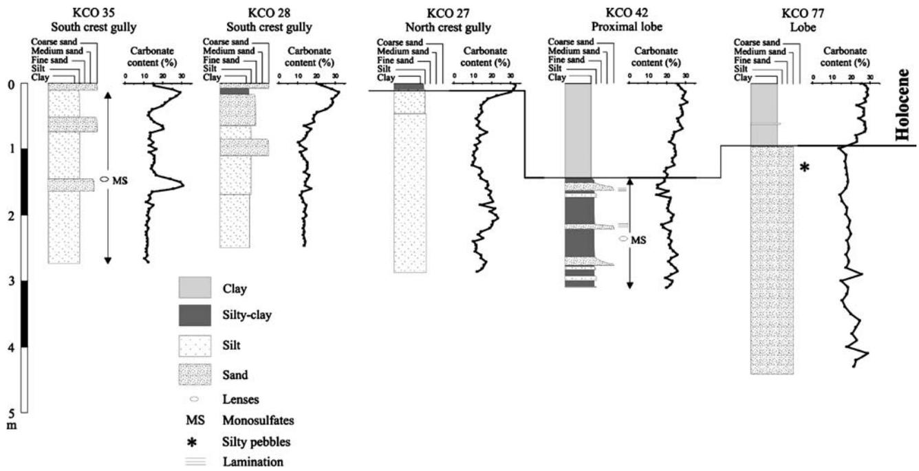
**Fig. 12** Core logs of the five cores collected in the Fium Alto gully and lobe, showing the main facies variations. Lateral correlation using carbonate content measurements is also shown (see Figs. 1 and 6 for core locations)
