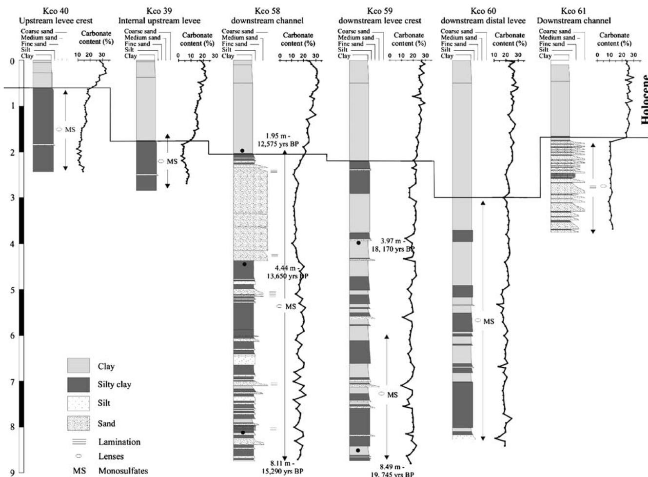
**Fig. 10** Core logs of the six cores collected in the South Golo channel–levee complex, showing the main lithologic facies variations. Lateral correlation using carbonate content measurements is also shown (see Figs. 1 and 6 for core locations)
