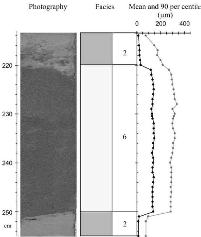
**Fig. 5** Photograph and grain-size curve showing structureless non-graded sandy sequence II: example from core Kcor 01 on the St. Damiano Levee (see Fig. 1 for core location)
