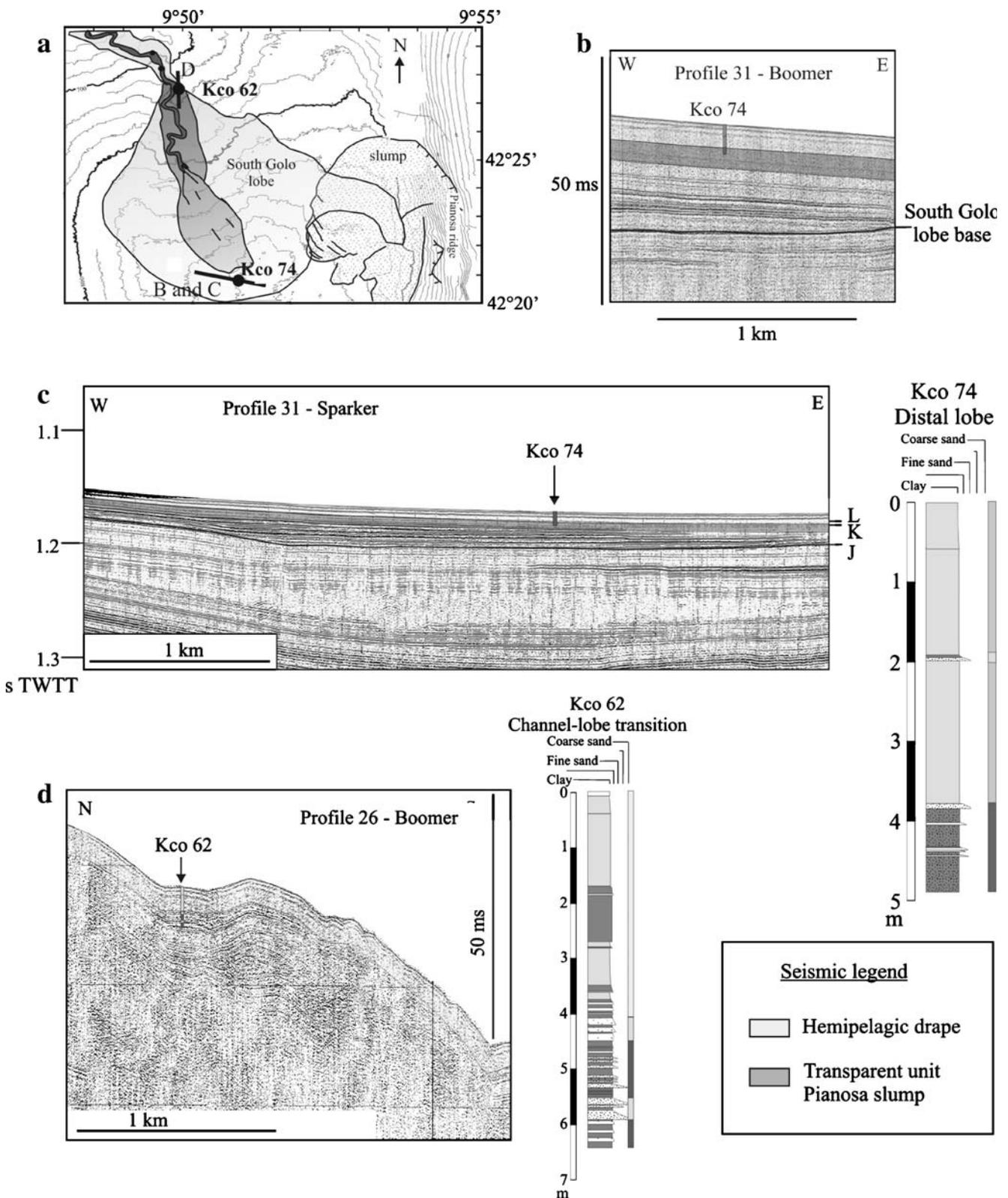
**Fig. 9** a–d Seismic profiles illustrating litho-seismic correlations for the South Golo lobe (a) boomer (b) and sparker (c) data for profile 31, and boomer data for profile 26 (d)
