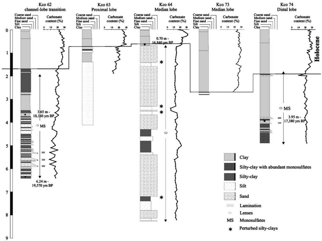
**Fig. 14** Core logs of the five cores collected in the South Golo lobe, showing the main facies variations. Lateral correlation using carbonate content measurements is also shown (see Figs. 1 and 6 for core locations)
