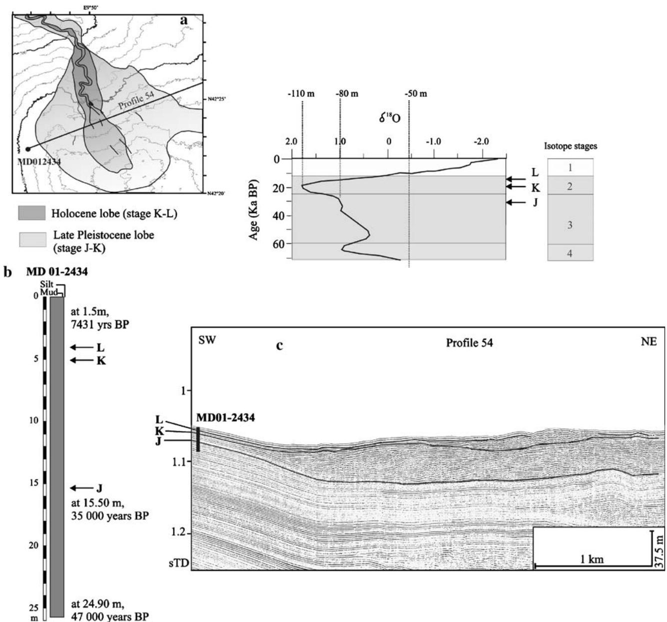
**Fig. 15** a–c Detailed bathymetric map of the South Golo lobe, showing a the locations of the seismic profile and core MD 012434, b the core log,  $^{14}\text{C}$  dates,  $\delta^{18}\text{O}$  isotopic curve, position of regional seismic markers J, K and L, and sea-level curve extrapolated from the model of
