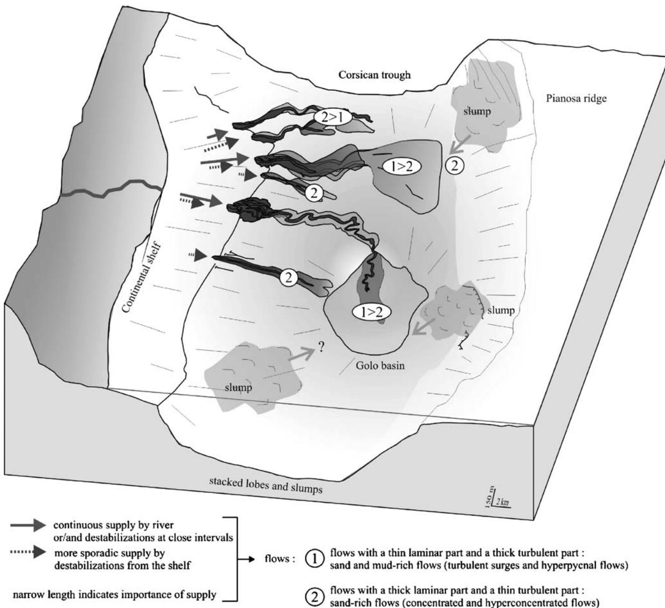
Fig. 16 Schematic representation of flow types along the Golo Margin. Arrow length is proportional to the relative importance of a given process
