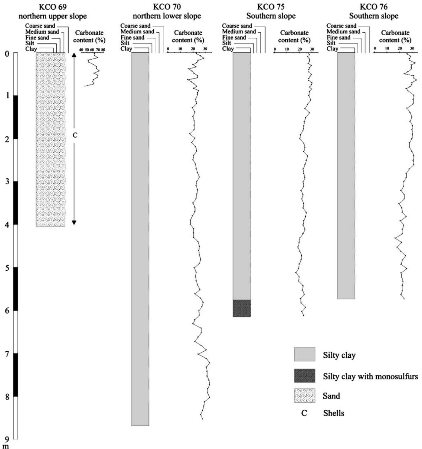
**Fig. 8** Core logs of the four cores collected on the Pianosa Ridge, showing the main lithologic facies variations (see Fig. 6 for core locations)
