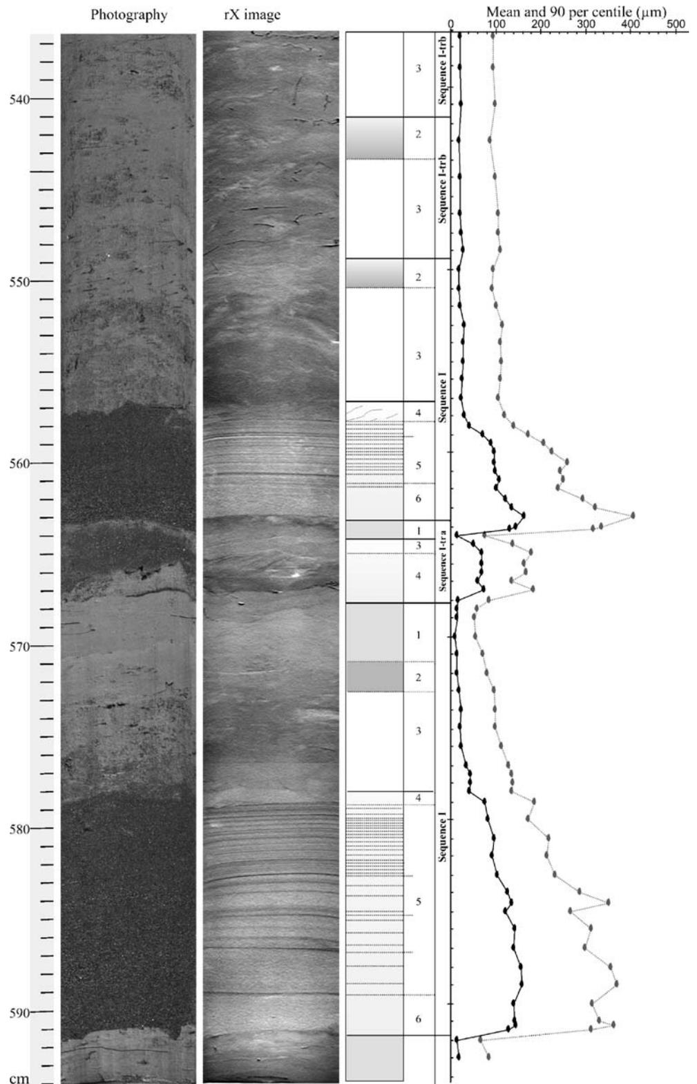
Lobes are characterised mostly by massive coarse sand (sequence III; Figs. 13 and 14) associated with chaotic seismic facies (Fig. 7). Numerous sequences I-tr are observed in the small, South Golo secondary channel lobe
