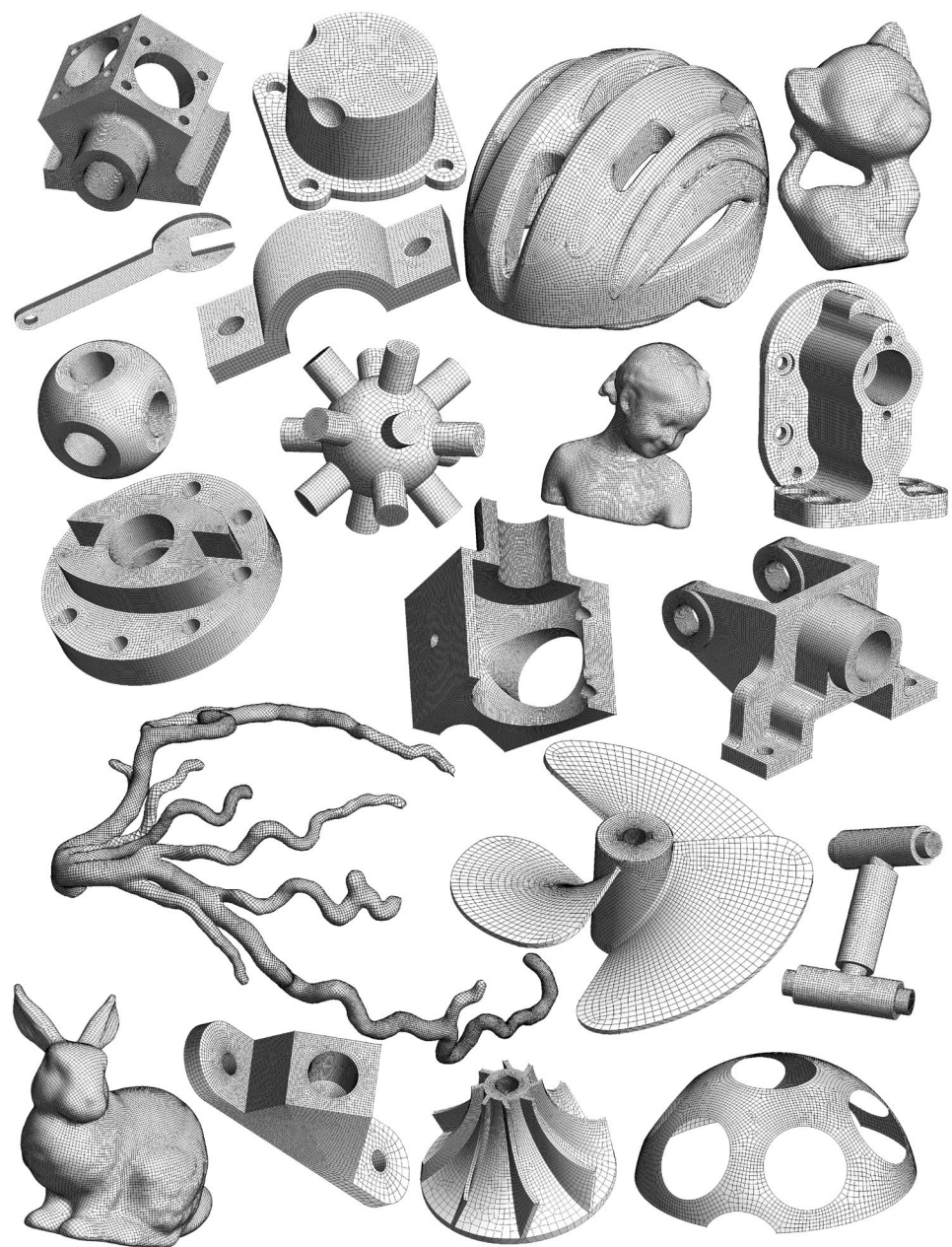
Fig. 12 All-quad meshes on various models obtained from the following sources: ABC [48], MAMBO [49], Thingi10k [50] and LoopyCuts [51]
