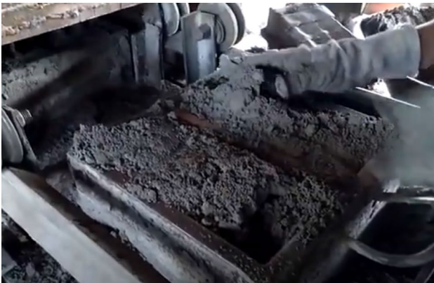
Fig. 9 Molding the mixture of fly ash and cement
