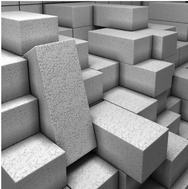
Fig. 14 Light weight fly ash bricks to save energy and cost reduction
