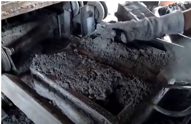
Fig. 12 Molding the mixture of fly ash and cement to produce light-weight bricks
