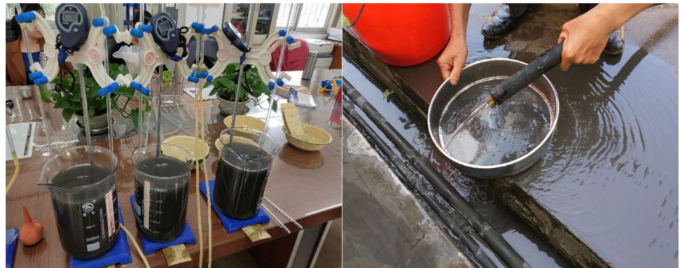
Fig. 2 The particle size test of raw tailings by gravitational and filtering methods
