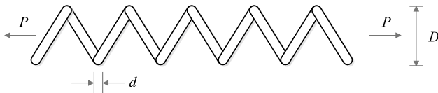
Fig. 11 Schematic view of tension/compression spring problem
