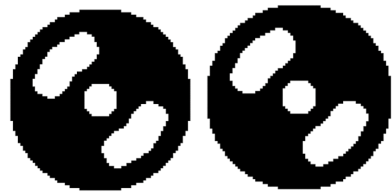
(a) Single-precision GPU symmetry constraint (b) Double-precision GPU symmetry constraint Fig. 19 Final topology found using the single-precision and double-precision GPU-LBM BESO algorithm with a symmetry constraint for the vorticity maximization problem
