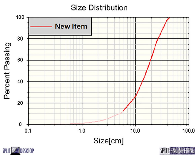
Fig. 1 Sample of a size distribution curve obtained using Split Desktop software
