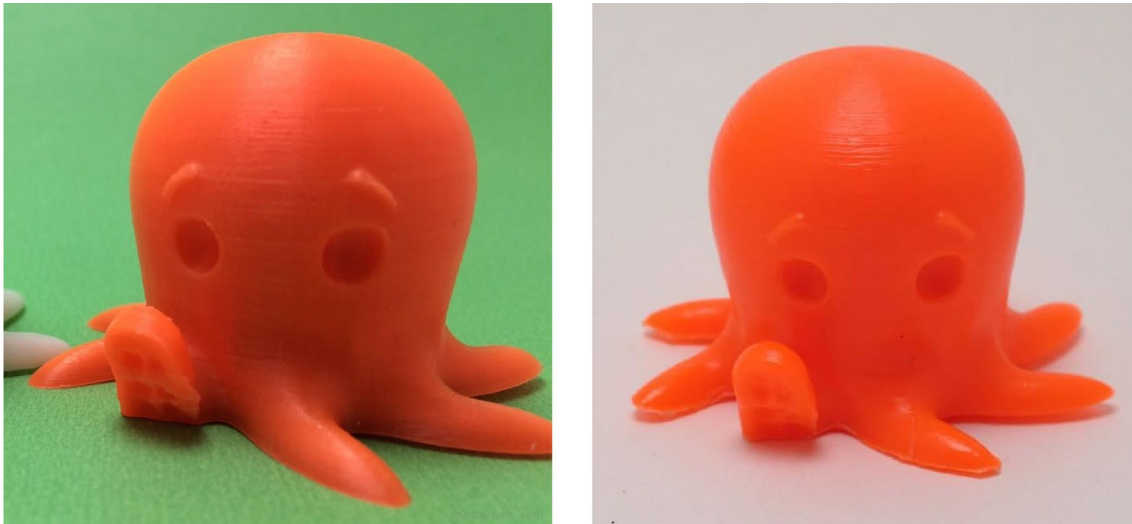
Fig. 5 FDM printed part before ( left ) and after ( right ) acetone finishing (courtesy of fabsterdam.com)
