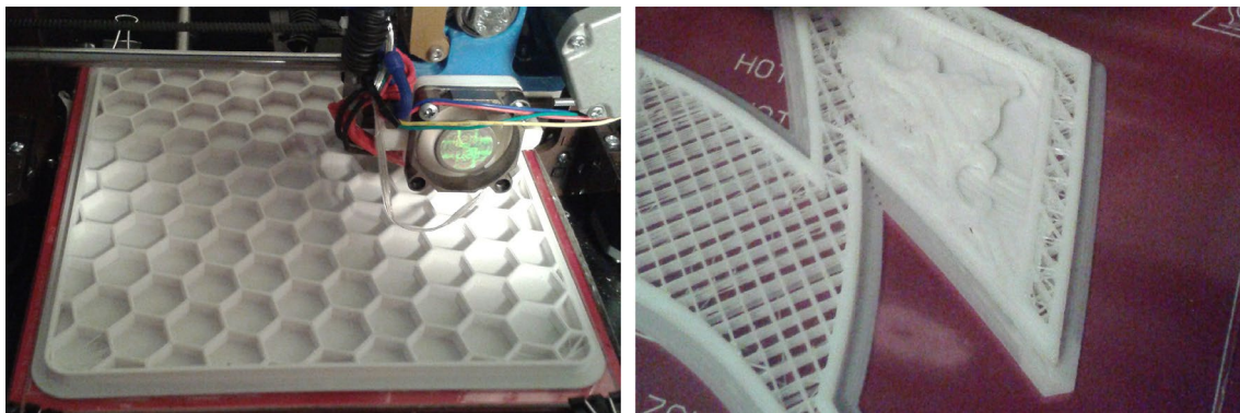
Fig. 1 Examples of Honeycomb ( left ) and Latticework ( right , courtesy of Aztec Scenic Design)
