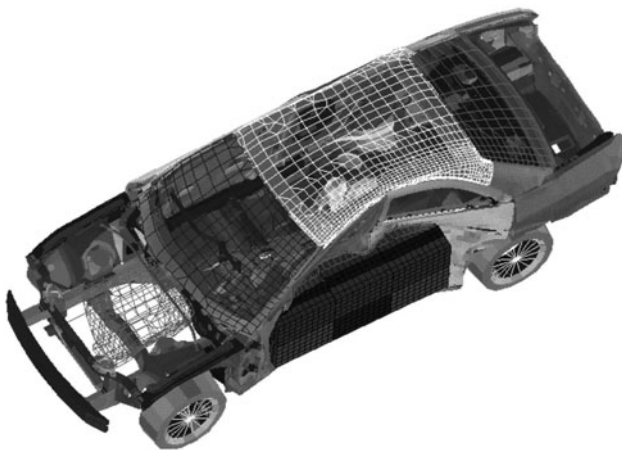
Fig. 16 Car side impact model [82]
