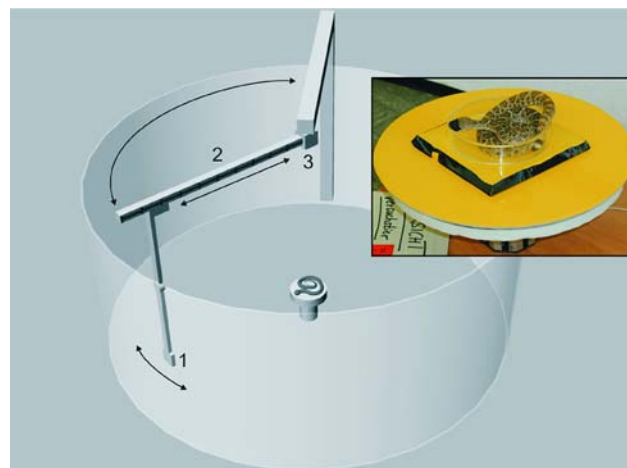
Fig. 1 Schematic sketch of the experimental setup. 1 IR source (Peltier element), 2 scale (100 cm), 3 perpendicular (not shown). Arrows indicate the moving directions of the platform. Inset shows blindfolded snake on the platform
