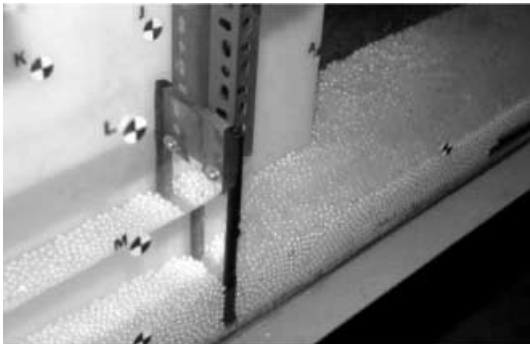
Fig. 15. Dam-break wave over granular bed experimental set-up installed at the Hydrotech Research Institute of the National Taiwan University. Shown are the initial conditions before removal of the sluice gate
