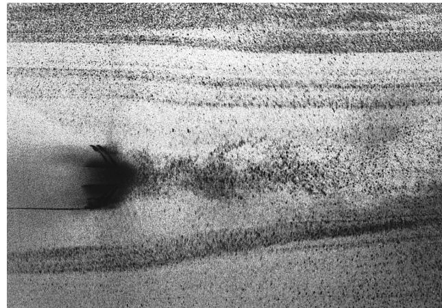
Fig. 3. A part of a PIV recording at Ma_2 = 1.27 with the model contour on the left hand side
