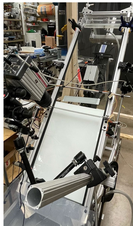
Fig. 2 Photograph of the falling film facility
