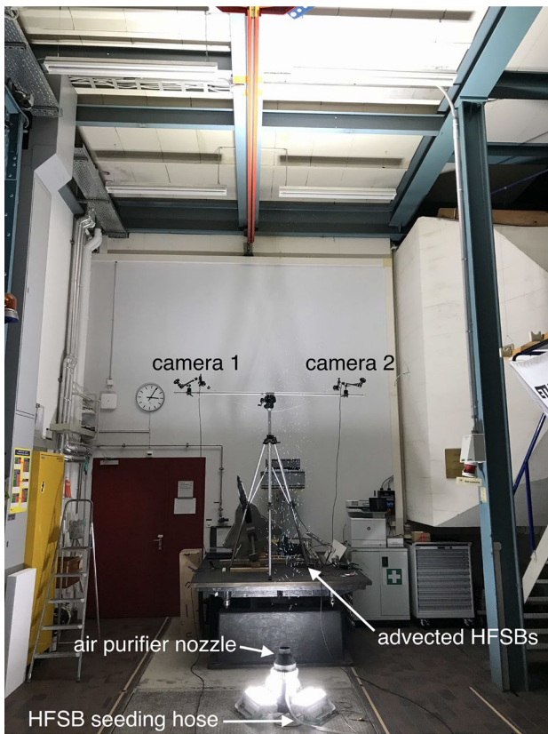
Fig. 4 TrackAER setup for the investigation of a large turbulent round free jet
