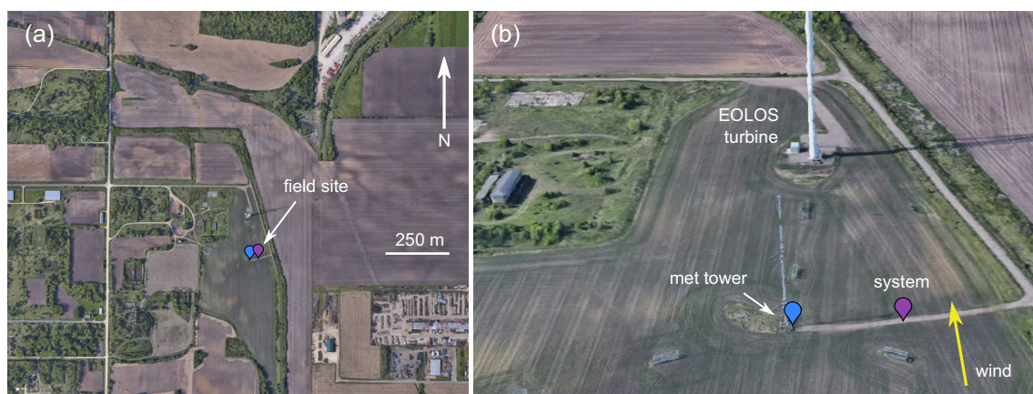
Fig. 5 Satellite images of field site for experiments in Rosemount, Minnesota, indicating positions of the system deployment in April 2022 and of the meteorological tower, as well as the mean wind direction from the deployment
