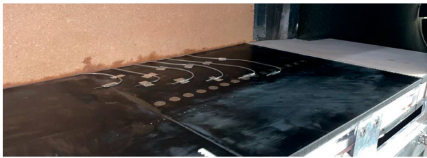
Fig. 2 The aft end of the flat plate setup mounted in the wind tunnel showing the staggered row of Preston probes
