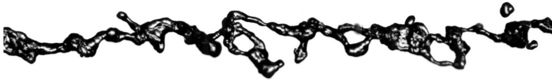
Fig. 19 Stitched image of a water jet originating from a 4 mm convergent nozzle with two 90° deflections upstream the nozzle entering (convU) at L/d_N = 167 and Re_{d_N} = 59,600
