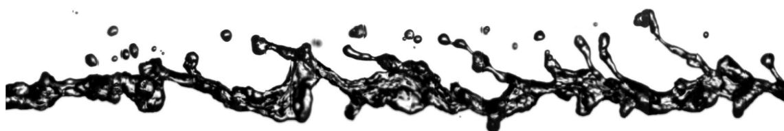
Fig. 18 Stitched image of a water jet originating from a 4 mm convergent nozzle with two 90^\circ deflections upstream the nozzle entering (convU) at L/d_N = 100 and Re_{d_N} = 59,600 . The imperfect stitching of the formed droplets due to their lower velocity is clearly visible
