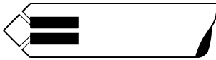
Fig. 7 Sketch of the two-hole pressure probe. The front diedral makes an angle of 90^\circ . The two pressure sensors are inserted inside the core of the probe
