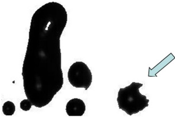
Fig. 9 A secondary droplet with a composite structure of ice and water, which appeared during rebound of a supercooled drop on a SHS at 0 °C
