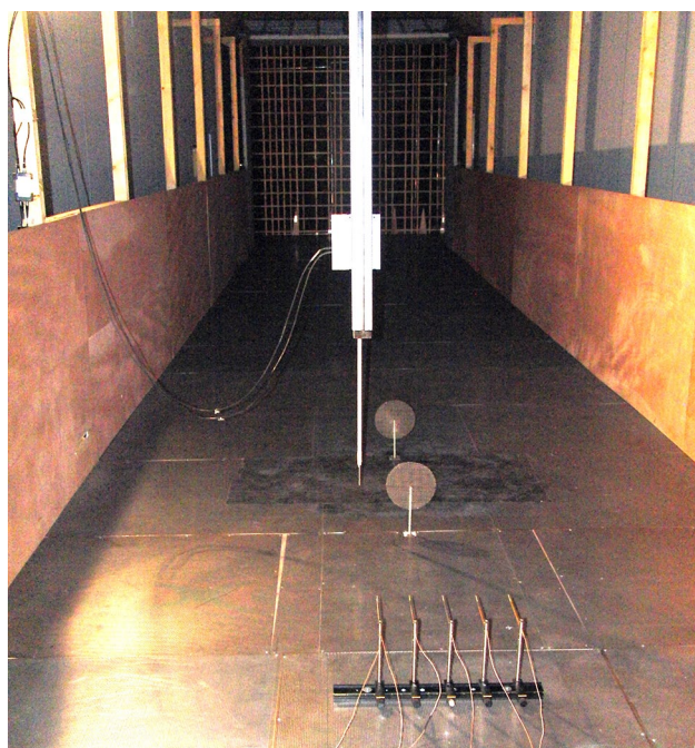
Fig. 7 Photograph of the experimental set-up (case 7). The traverse system holds the upstream hot wire, and may be moved in front of the hub of the downstream turbine during the acquisition
