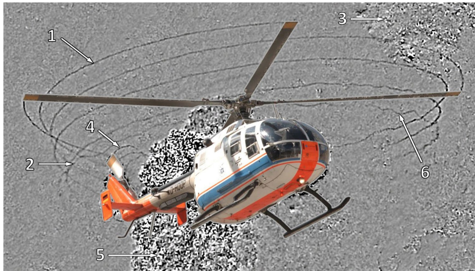
Fig. 4 Photograph of the BO 105 during a swinging maneuver, acquired by camera 2. The displacement gradient field is overlaid, depicting the tip vortex positions
