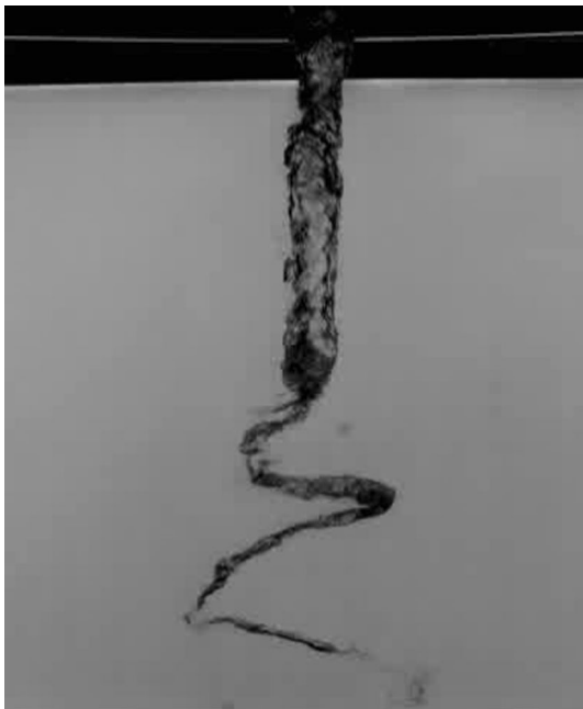
Fig. 1 Photography of a Francis turbine vortex rope, EPFL laboratory for hydraulic machines
