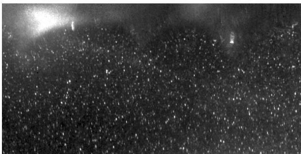
Fig. 3 PIV image with a deformed free surface. Contrast has been enhanced. The interface cannot be directly and accurately found because of the distorted reflections and refractions. An internally reflected beam can be seen on the left of the image
