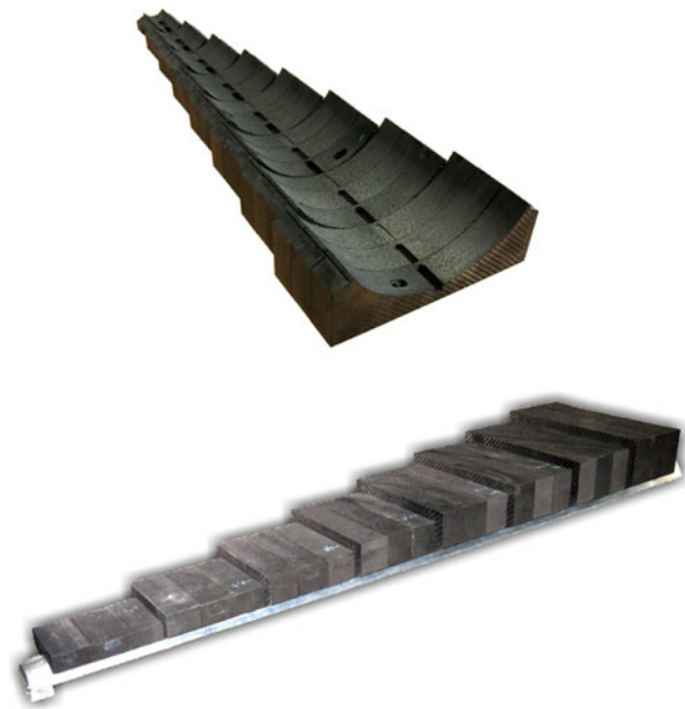
Fig. 8 Single CNC milled C/C parts ( top ) and model insert with bonded ceramic parts ( bottom )
