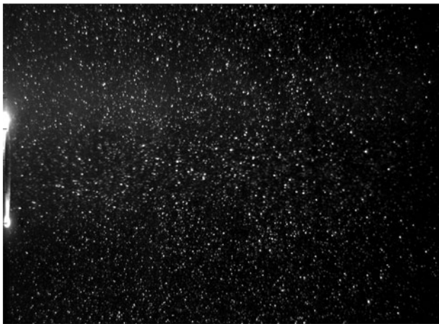
Fig. 4 Sample streamwise PIV image at Re = 10,000 . Pipe outlet is visible at the far left of the picture
